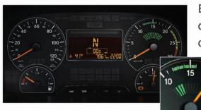
Eco meter indicator gives indication to the driver on the correct gear and speed for optimum fuel efficiency.
